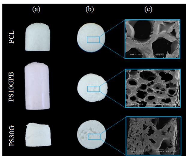
**Figure 1:** Selected images of samples prepared by SFM (for 2 h, 20 MPa, 40 °C and 0.37 L<sub>CO2</sub>·min<sup>-1</sup>). (a) Side-view; (b) Top-view and (c) SEM micrographs for pure PCL, and for PS10GPB and PS30G biocomposites.
