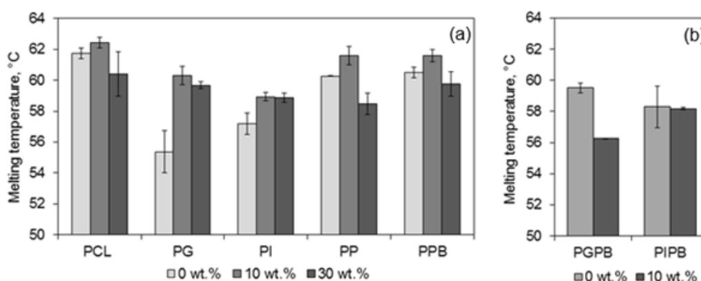
**Figure 2:** Melting temperatures of samples prepared by SFM (for 2 h, 20 MPa,  $40^\circ\text{C}$  and  $0.37 \text{ L}_{\text{CO}_2} \cdot \text{min}^{-1}$ ). (a) single liquid additive; and (b) mixture of two liquid additives. Biocomposites were prepared with different SNPs amounts (0%, 10 and 30% w/w).
